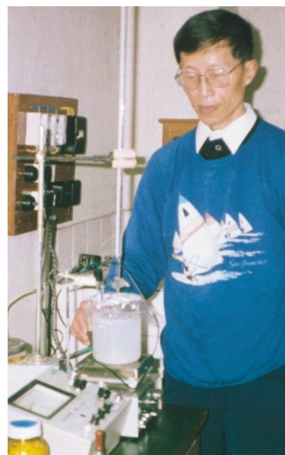
Dr Guo carrying out a precipitation experiment on the effluent from an acrylic acid plant at Shanghai Jiao Tong University
